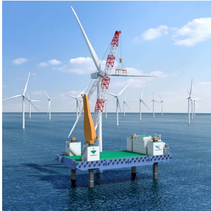
Project 05 SEP (Self Elevating Platform) Image
